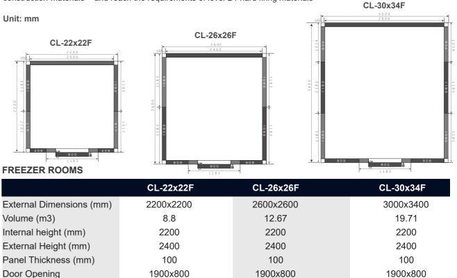
External Dimensions (mm) Volume (m3) Internal height (mm) External Height (mm) Panel Thickness (mm) 1900x800 Door Opening
